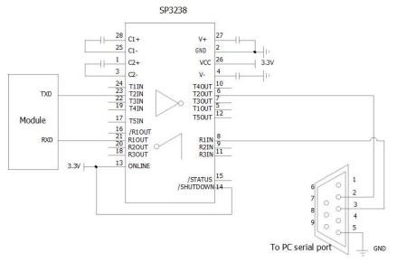
Figure 5: RS-232 Level Shift Circuit
