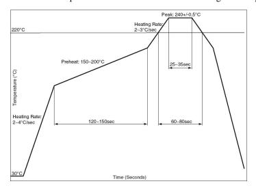
Figure 9: Recommended Reflow Soldering Thermal Profile
