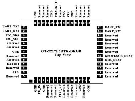
Figure 3: Pin Assignment
